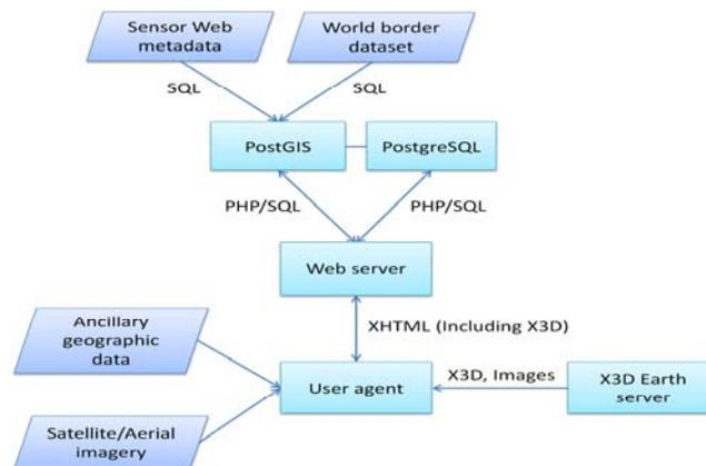
Figure 1. Data, application and communication technologies used in the proposed system.
